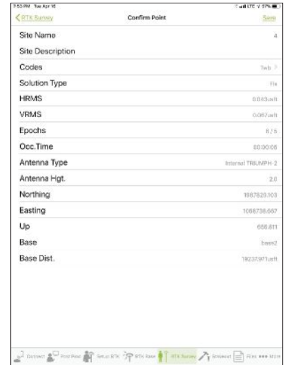
POINT CONFIRMATION Survey point information with metadata and equipment listing.
