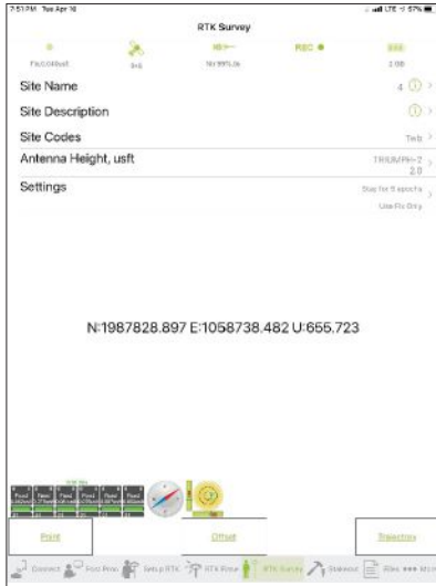
IOS POSITION Status of survey data collection and GNSS engine signal reception.
