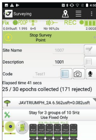
SURVEY POINT Status of survey data collection and GNSS engine signal reception.
