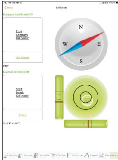
RECEIVER SETUP Visual reference for leveling and direction of GNSS receiver.
